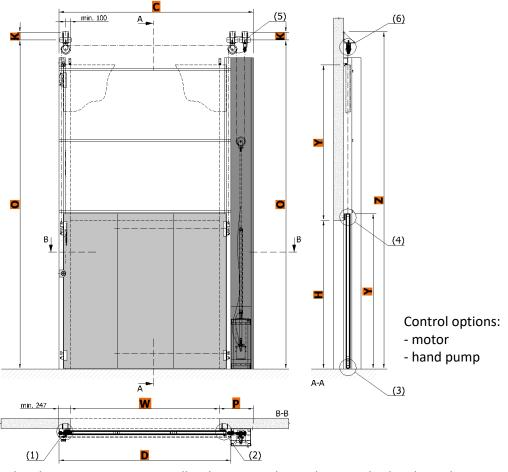
Minimum height H<sub>min</sub> = 2000 mm. Smaller dimensions has to be consulted with producer.
