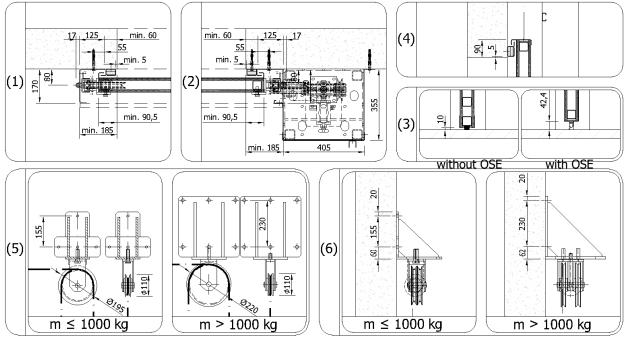
Minimum required dimensions of steel structure
