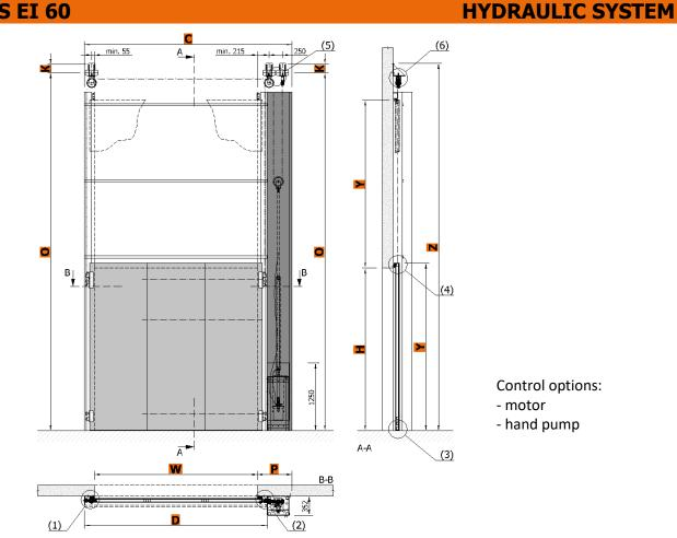
Minimum height H<sub>min</sub> = 2000 mm. Smaller dimensions has to be consulted with producer.
